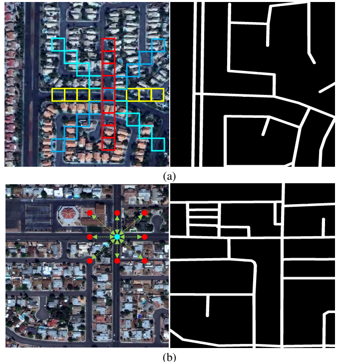
Fig. 1: Motivation of the strip convolution module and the connectivity attention module that we proposed. From left to right: satellite imagery, ground truth. (a) Strip convolutions with four shapes are used to capture linear features of roads. (b) Connectivity of one pixel with neighboring pixels is predicted to capture local pair-wise dependencies and ensure road topological correctness.
