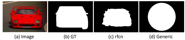
Figure 24 Failure Case. Our S-measure ranked (d) Generic higher than (c) rfcn due to these prediction map without obvious structure.
